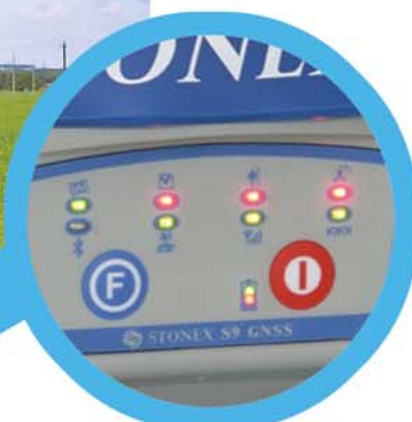
New front panel with indicators led for individual functions to indicate the status of receiver
